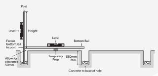
For first module, position bottom rail to suit length of slats. Secure bottom rail to post using 10x16 tek screws on either side of post. When installing LYSAGHT SLATSCREEN™, the bottom rail should be installed inverted, with the opening in the rail facing downward towards the ground.
