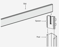
Insert slat spacers into front portion of the post, one at each end at a time. Drop slat down into spacer and repeat process, building the slats to the full height of the posts.\*
