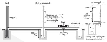
Secure 2 posts back-to-back, allowing for step if required. Continue to fix bottom rails to posts, place in a hole, brace posts and level bottom rails.
