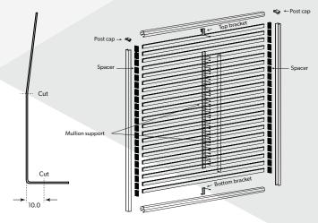
Locate two mullion brackets. Cut ONE of the brackets as shown on drawing above - this bracket is to be used to secure the mullion to the bottom rail. Locate mullion bracket mid-way along panel and secure one half of the mullion to the brackets, use #8x12 button head screws to secure mullion to slats - 2 per slat. Place other half of mullion over the first to conceal fixings and secure with pop rivet(s).
