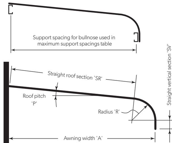
$$\left. \begin{array}{l} \text{Span to be used in} \\ \text{determining wind pressure} \\ \text{capacities of bullnoses} \end{array} \right\} = SR + (\text{arc of radius } R)$$
